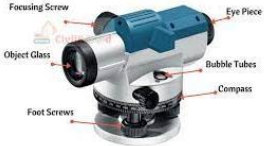
Components of Dumpy Level
